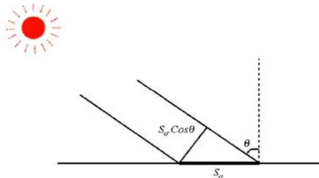
Fig. 2.3 Angle of incidence  $\theta$  of the solar radiation [7].
