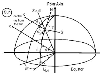
Fig 2.2. Schematic representation of the solar angles [7]
