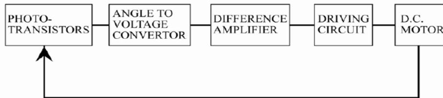
Fig 4.6 Block diagram of sun-tracking system [61]
