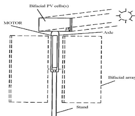
Fig. 4.2. Scheme of the terrestrial tracker [40].
